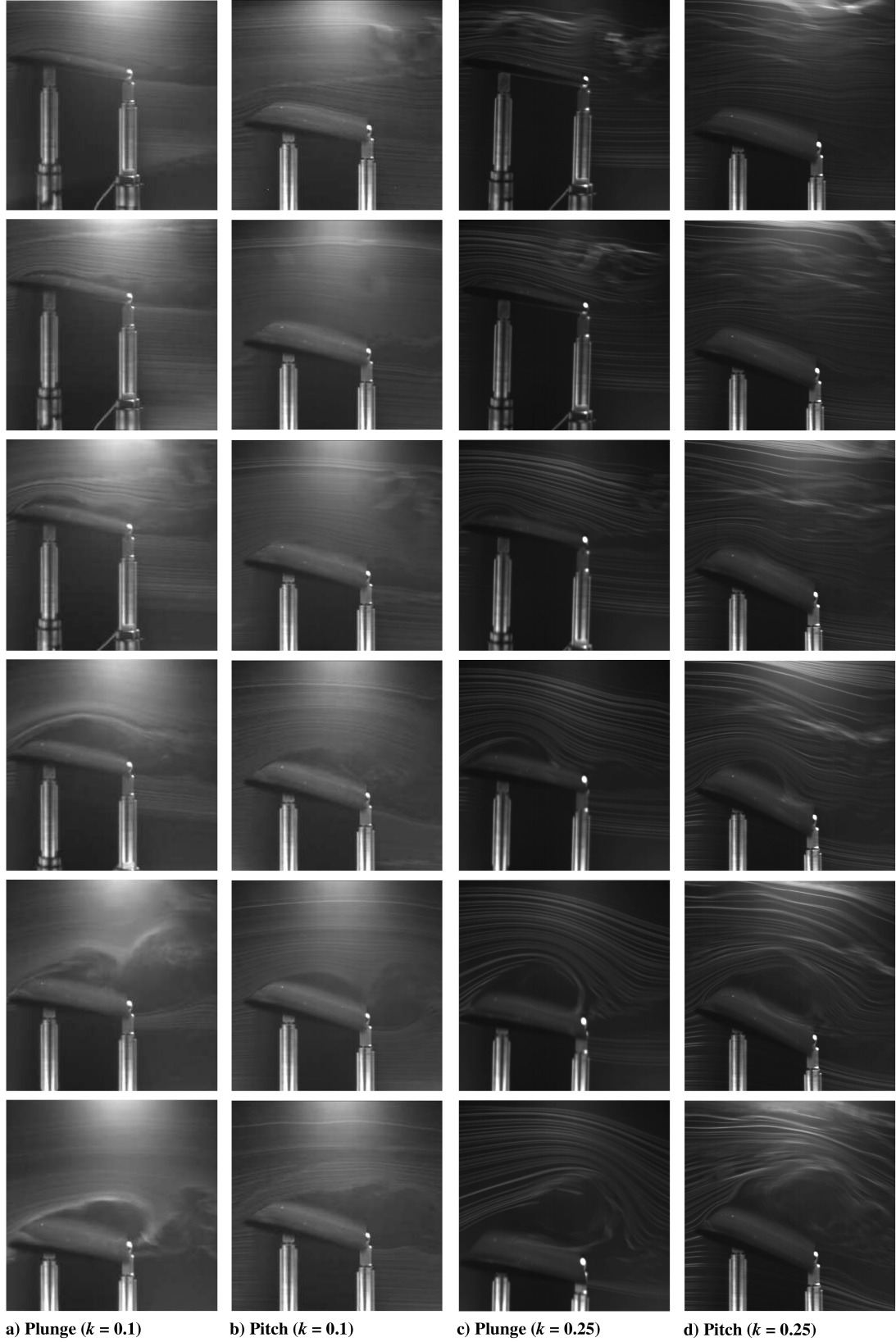
Fig. 5 Comparison of equivalent pure-plunging and pure-pitching kinematics using smoke visualization with a mean angle of attack of \alpha_o = 8^\circ . Note that sequences start at t/T = 0 (top of stroke) and follow in constant steps of t/T = 1/16 . For k = 0.1 the effective angle of attack varies from top to bottom with \alpha_{\text{eff}} = 8, 10.2, 12.1, 13.3, 13.7 , and 13.3^\circ ; for k = 0.25 , the variation is \alpha_{\text{eff}} = 8^\circ, 13.5, 18.1, 21.1, 22.1 , and 21.1^\circ .
